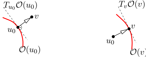
Figure 2.2. Minimizing the distance of v to \mathcal{O}(u_0) (left) or of u_0 to \mathcal{O}(v) (right).
