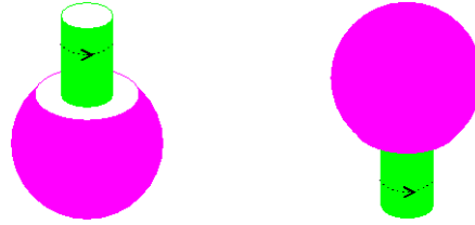
Figure 1.1. From left: a sketch of the noninverted and inverted states of the tippe top.
